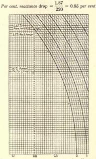
Fig. 131.—Illustrating the application of the Mershon diagram for computing a three-phase, three-wire alternating-current circuit.
